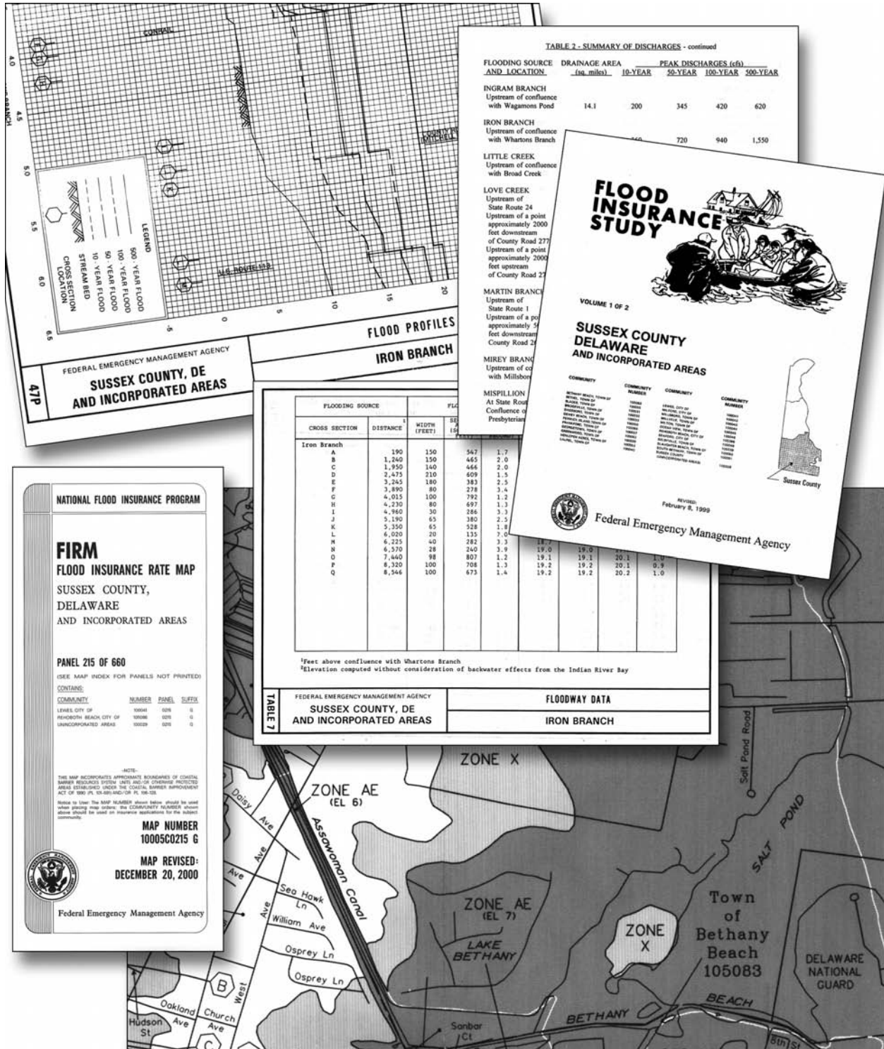
Figure 4-1. Portions of an FIS and a FIRM.
